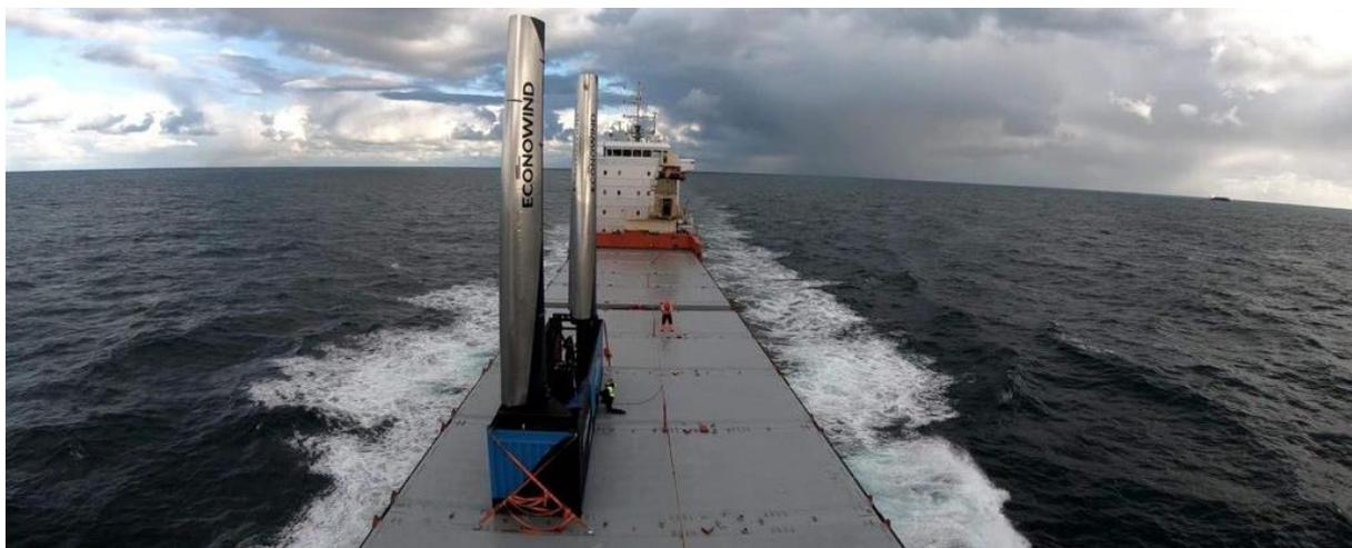
*One eConowind unit mounted on the hatchcovers in testphase.*
