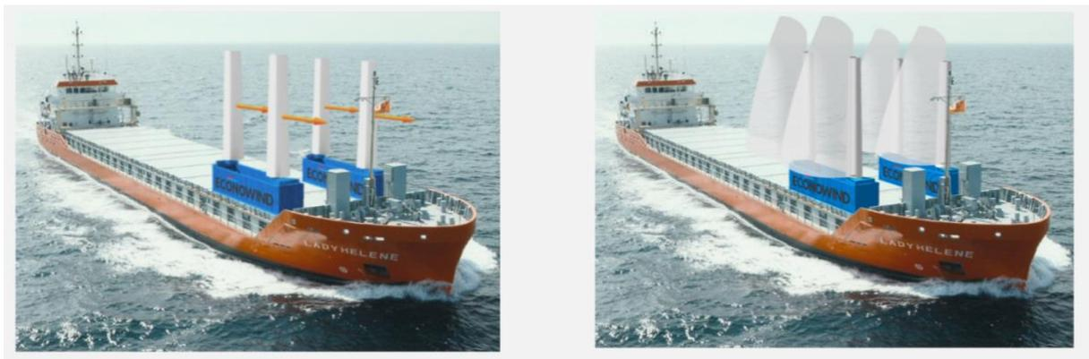
*For equivalent thrust force of two eConowind-units, a sail area of abt. 165 m<sup>2</sup> should be applied*
